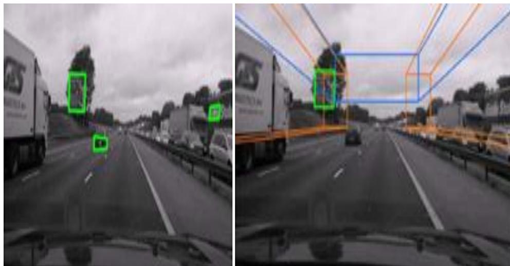
Figure. 1. System output showing detection of traffic signs (left) without and (right) with the use of structural and temporal information
